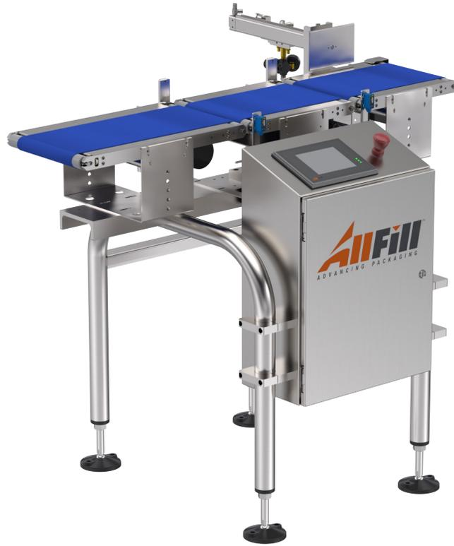
The Model EW-8 is All-Fill's economical solution for users and applications that may only require an entry level checkweigher. The EW-8 offers 0.5g resolution. It utilizes a strain gauge load cell for weighing packages up to 5 lbs and operating at speeds up to 120 packages per minute, this makes the EW-8 just as versatile and reliable as other All-Fill models.
