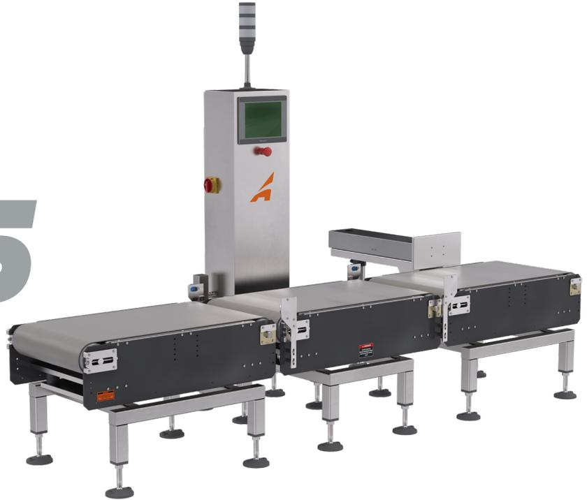
All-Fill HW-15 Checkweighers are heavyweight models capable of handling large size cases, bags, and packages, up to 42 inches in length and 24 inches in width. They can operate at speeds up to 50 containers per minute and handle packages weighing up to 200 lbs. Featuring a Four Point load cell design, the HW-15 can weigh with an accuracy of  $\pm 0.25$  oz, depending on the application. Reduce waste and increase accurate production with a heavyweight checkweigher from All-Fill.
